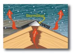
Engineered from a unique corrugated plastic material, Trimline vents fit a variety of roof styles including shingle, cedar, tile and metal. Designed to vent at the ridge - the hottest point of the roof - the Trimline vent system has the added benefit of creating a smooth roofline, eliminating the unsightly louver vents commonly found on many homes.
